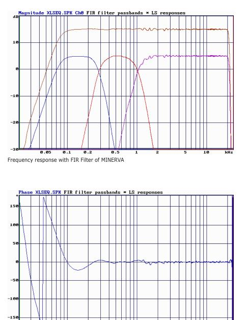
Phase response FIR linear phase Filter of MINERVA
